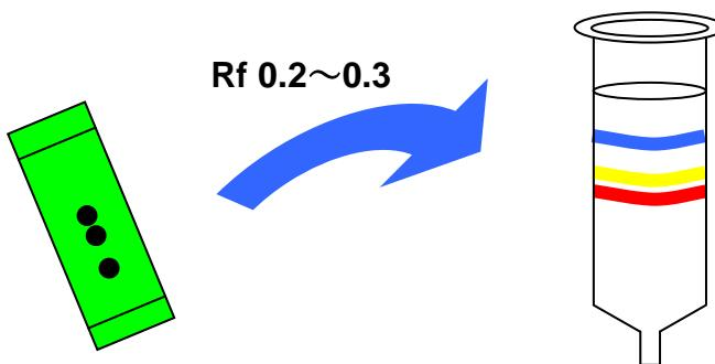
When running samples with the solvent mixture ratio (solvent strength) that moves samples at Rf0.2 - 0.3 (0.25 on average) TLC, it is a proven fact that good separations are achieved in the normal phase silica column chromatography. Rf0.2 - 0.3 is equivalent to 3.3 – 5 CV (4 CV on average). Chemists used to run the TLC several times in conventional chromatography to get the solvent mixture ratio that gives Rf0.2 - 0.3. It was a very time-consuming job.
